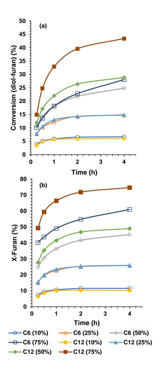
**Figure 2.** (a) Conversion of diols to furan-esters (expressed in mol %) during oligomerization, determined *via* <sup>1</sup>H NMR. Medium: diphenyl ether, N435: 20% w/w, temperature: 100 °C. (b) Composition of copolyesters during oligomerization showing the evolution of furan content in
