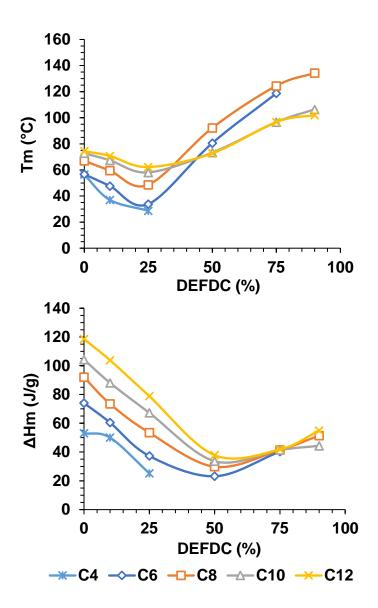
**Figure 3.** Variations in melting endotherms (°C) and crystallization enthalpies (J/g) as a function of diol length and furan content.
