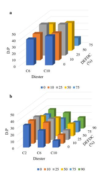
**Figure 1.** (a) the variation in DP of furan-based copolyesters with variable furan content based on hexane-1,6-diol and different aliphatic diesters. (b) the variation in DP of furan-based copolyesters with variable furan content based on dodecane-1,12-diol and different aliphatic diesters, where  $(C_2=1,2$ -diethyl oxalate),  $(C_6=1,6$ -diethyl adipate), and  $(C_{10}=1,10$ -diethyl sebacate).
