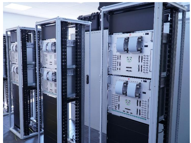
Figure 2. HiL testbeds with HIL real time simulators and hardware signal interfaces
