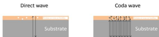
Fig. 1. Schematic illustration of ultrasound wave propagation in the medium: direct waves (left) correspond to first reflected and backward propagated echoes, whereas coda waves (right) are multiply reflected and scattered inside the medium when a change at solid interface of substrate occurs.
