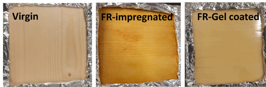
Fig. 4. Images of the wood without coating (virgin), after immersion in sol-gel solution (FR-impregnated) and after sol-gel coating with a spatula (FR-gel coated).
