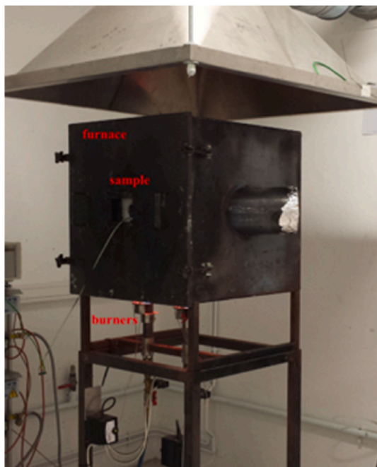
Fig. 2. Image of the small furnace fire test 10 cm*10 cm.
