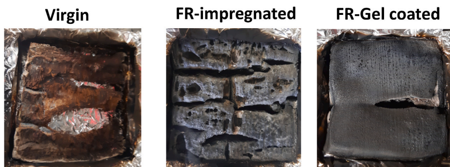
Fig. 7. Digital pictures of the chars of the virgin, FR-impregnated and FR-gel coated wood samples.
