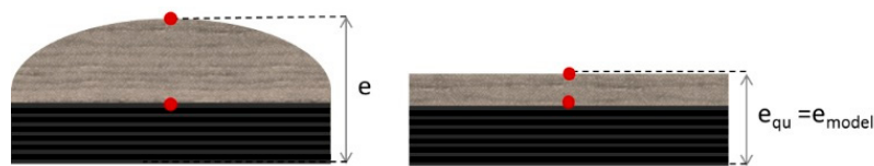
Figure 10. Scheme of the determination of the equivalent thermal conductivity with a volume constant assumption [6].
