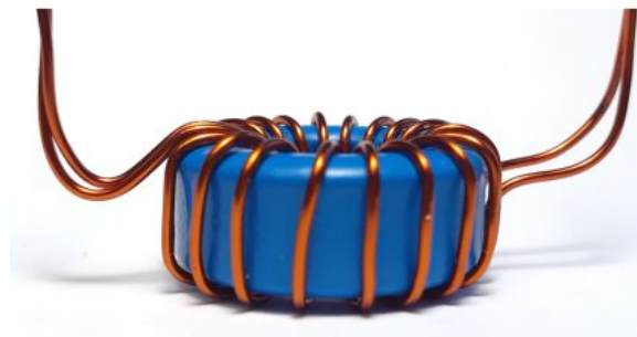
Figure 2. Toroidal core with two windings-side.
