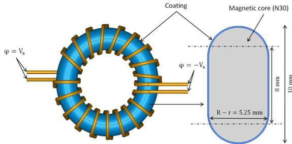
Fig. 7. 3-D model of the transformer.
