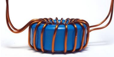
Fig. 6. Toroidal core with two windings.
