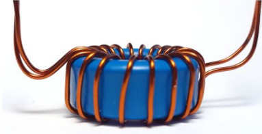
Fig. 6. Toroidal core with two windings.
