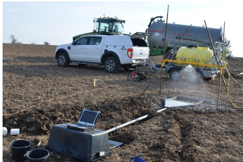
Figure 3. Rain simulator: a frame having a nozzle and an assembly for sampling water runoff.
