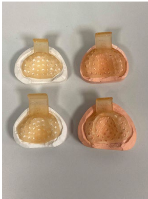
Figure 6. Four 3D-printed impression trays fitted to their gypsum casts.
