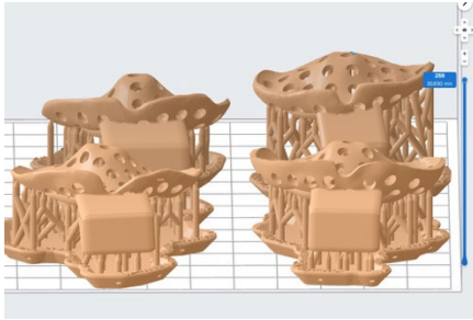
Figure 5. Preparation for printing TS21 infant-specific impression trays using Preform software program (Formlabs).
