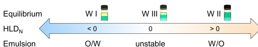
Figure 2. Illustration of SOW systems behaviour with HLD_N evolution when emulsified (bottom) and at equilibrium (top).
