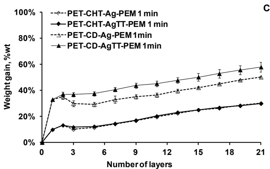
*Figure 2: Weight gain of textiles after pad/dry/cure step with citric acid and CHT or CD (layer #1), silver sulfate loading with or without Thermal Treatment (layer #2), and n cycles of layers depositions by L-b-L process in CHT solution (0.5% w/v) and in polyCTR-βCD solution (0.3% w/v) with dipping times of 1, 5 and 15 minutes.*
