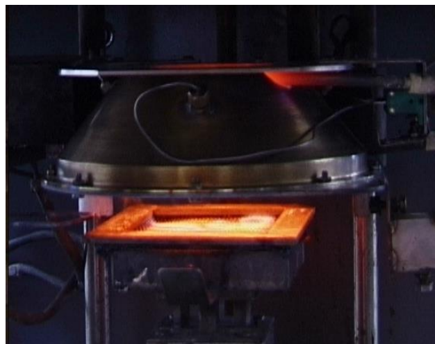
Figure 37. Fire behavior of M5 when subjected to 75 \text{ kW/m}^2 [126]
