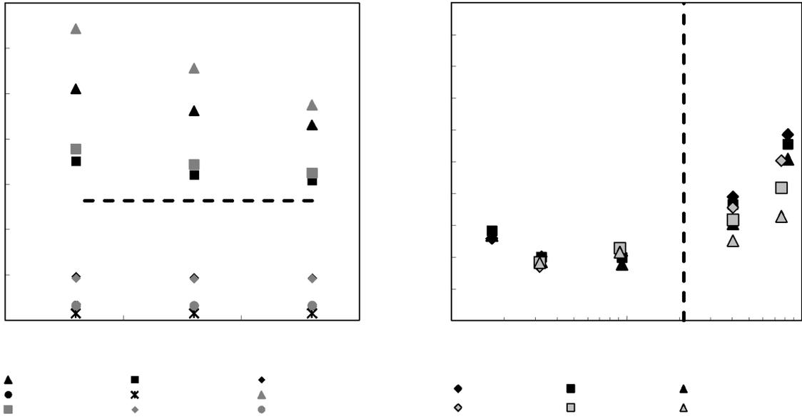
**Figure 3.** A) Permeate DPC concentration vs. trans-membrane pressure, at different retentate concentrations “Co”. Gray and Black symbols represent 15 kDa membrane and 5 kDa, respectively. B) DPC retention at different DPC retentate concentrations Co. Dotted line represents the CMC
