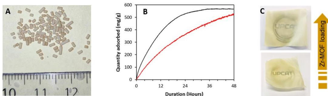
**Fig. 1** UiO-66-NH<sub>2</sub>@chitosan granules (A) and their relative iodine adsorption kinetic curve (B, red) compared to their powder counterpart (B, black). UiO-66-NH<sub>2</sub>@chitosan films with various MOF loadings (B).
