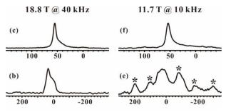
Figure 1. 1D <sup>27</sup>Al MAS NMR spectra of parent NH<sub>4</sub>-ZSM-5 (a and d), calcined and dehydrated H-ZSM-5 (b and e), TMPO-adsorbed H-ZSM-5 with P/AI = 0.42 (c and f), obtained at  $B_0 = 18.8$  T (a-c) and  $B_0 = 11.7$  T (d-f). The asterisks denote spinning sidebands.
