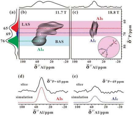
**Figure 4.** 1D one-pulse <sup>31</sup>P MAS (a) and 2D <sup>31</sup>P {<sup>27</sup>Al} PT-D-HMQC MAS (b) NMR spectra recorded at 11.7 T, and 2D <sup>27</sup>Al {<sup>31</sup>P} D-HMQC MAS NMR spectrum (c) recorded at 18.8 T of dehydrated H-ZSM-5 zeolite (Si/Al = 25) with adsorbed TMPO (P/Al = 0.42). Selected slices with simulations are shown on (d) and (e).
