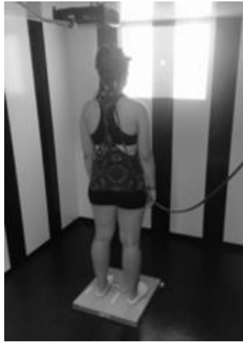
Figure 1. Experimental setup with a participant inside the moving room, standing on a force plate using the eye tracking device while performing the saccadic visual task.
