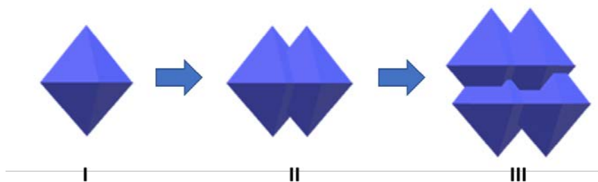
Figure 4: Schematic representation of the effect of concatenated growth of different MOF crystals: I) representation of a single crystal; II) interpenetration of 2 crystals and III) interpenetration of multiple crystals.
