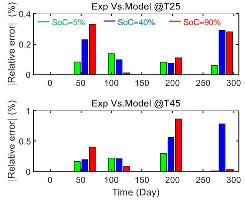
Fig. 2 Relative error on capacity for calendar aging
