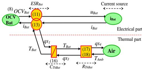
Fig. 9 EMR of the battery electro-thermal model
