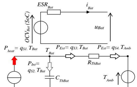
Fig. 8 Structure of the simplified electro-thermal model
