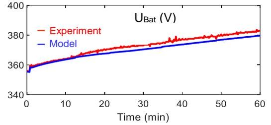
Fig. 11 Comparison of model and experiment for  $u_{Bat}$
