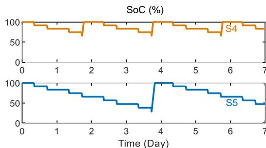
Fig. 16 Battery SoC evolution for different charging intervals
