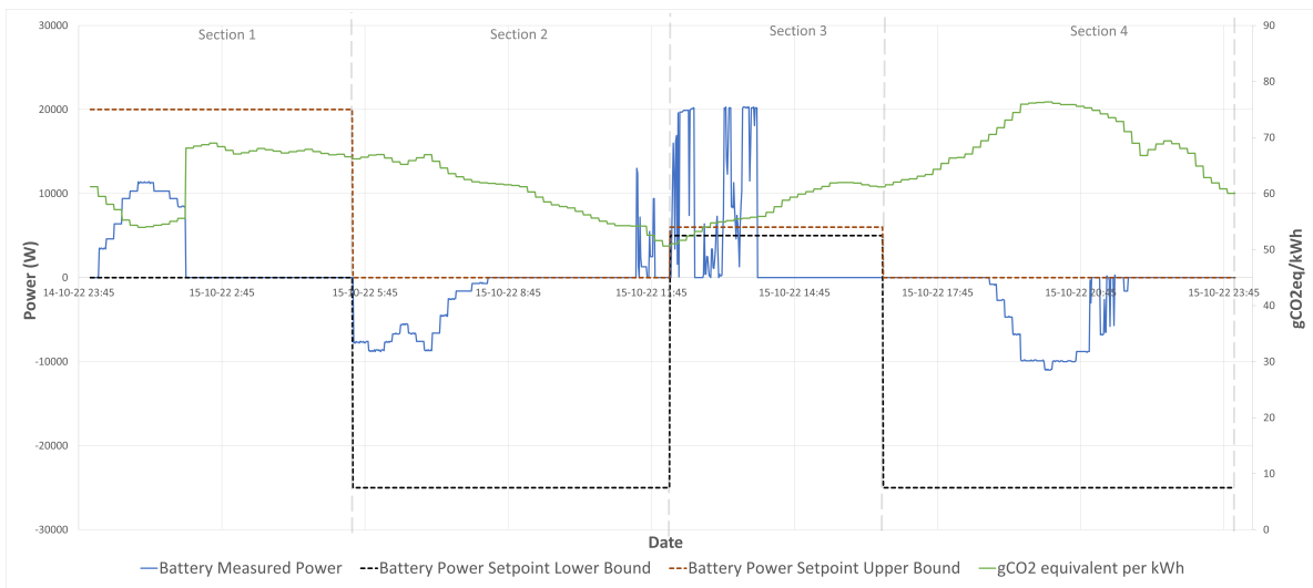
Figure 20: Battery setpoint power profile, grams of CO2 equivalent per kWh, battery setpoint lower and upper bounds for the 15 th of October 2022, four sections outline the different stages based on time and bounds
