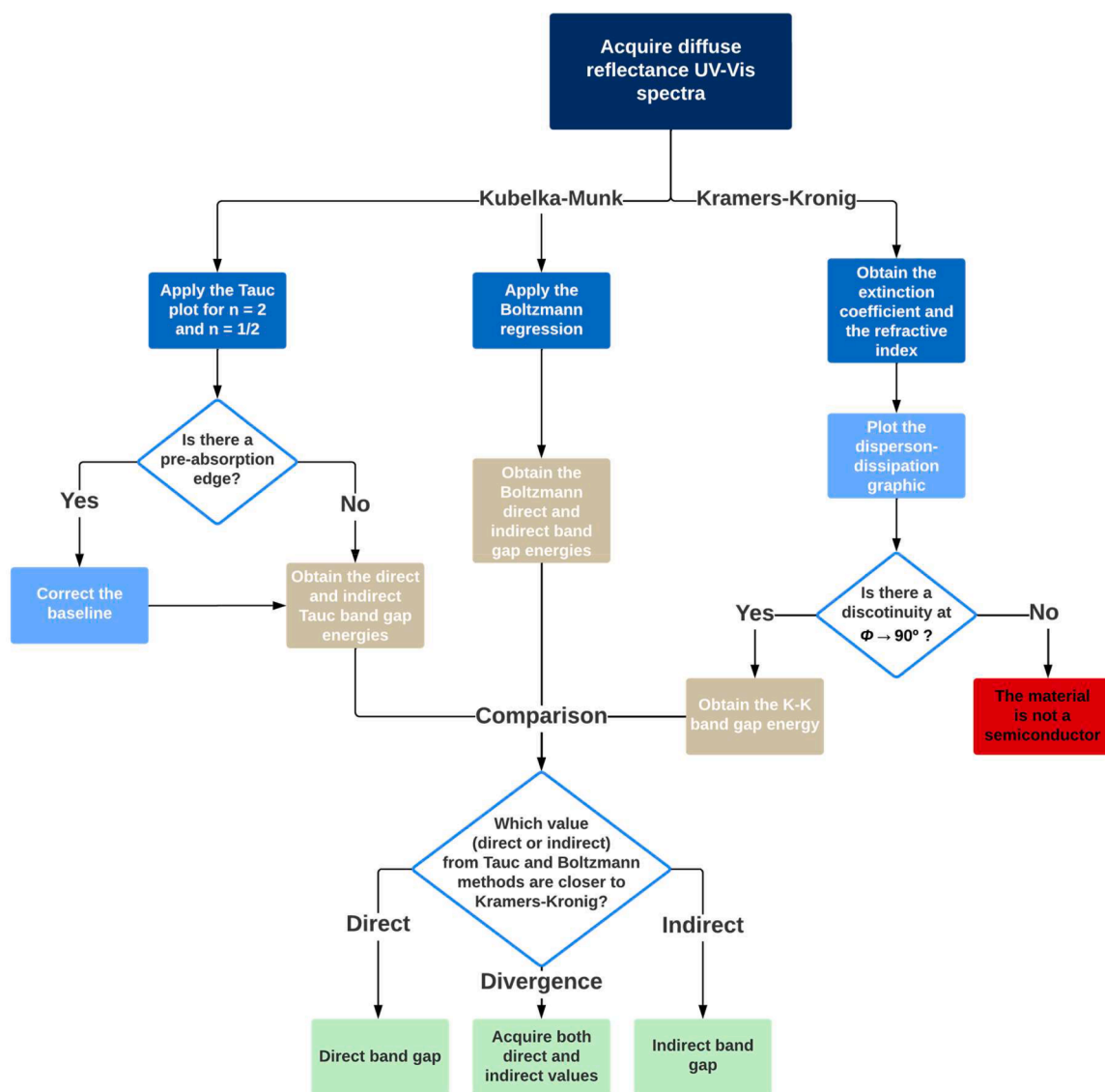
Fig. 11. Flowchart demonstrating the methodology for determining whether a material has a direct or indirect band gap transition.
