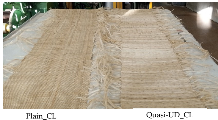
Figure 2. Woven and quasi-unidirectional fabrics.
