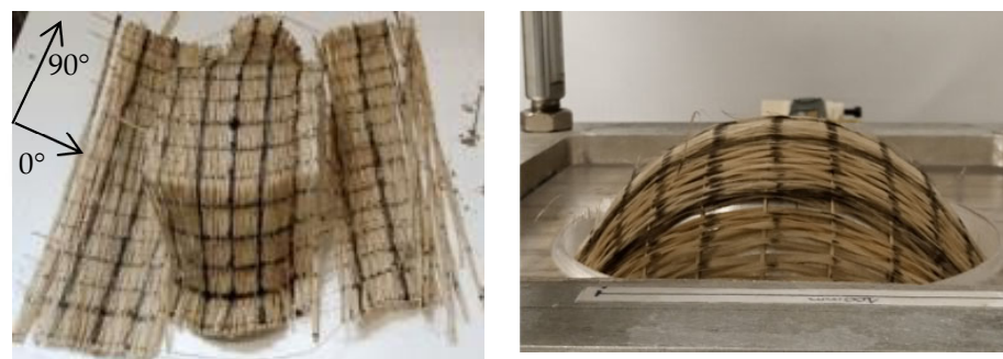
Figure 14. Defects on Quasi-UD_CL fabric after forming.
