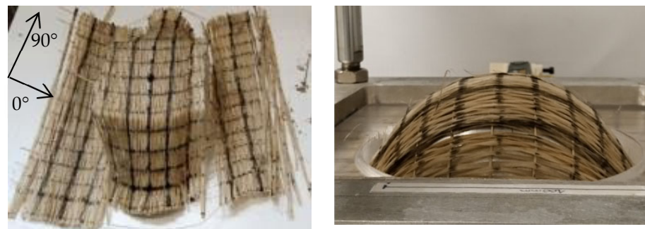
Figure 14. Defects on Quasi-UD_CL fabric after forming.
