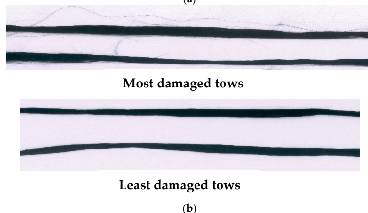
Figure 6. (a) Tension during rewinding process; (b) pictures of carbon tows after rewinding.
