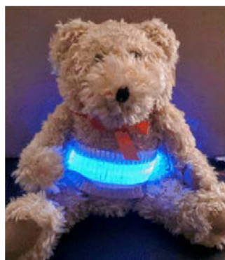
Figure 17. The fabric is wrapped around a teddy with 120 POF illuminated [95] (Reprinted with permission from Ref. [95]. Copyright 2021 Biomedical Optics Express).
