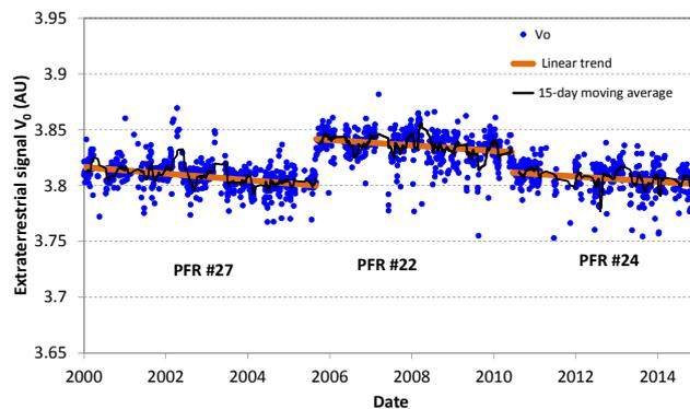
**Figure 4.** Daily extraterrestrial voltages ( $V_0$ ) at the 500 nm wavelength obtained with the Langley plot method for the GAW-PFR at Mauna Loa (morning calibrations only). The temporal linear fit to the  $V_0$ 's for each instrument deployment, as well as the 15-day moving average, is superimposed. Note that these are instrument signals; i.e., they depend on each particular instrument and are not directly comparable.
