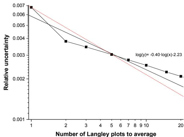
**Figure 6.** Uncertainty of the Langley plot calibration vs. number of Langley plot  $V_0$ 's that are averaged, using GAW-PFR data (500 nm) at Mauna Loa (2000–2014). The black line indicates the fit to the experimental data in log–log scale (fit result provided). The red dashed line indicates the theoretical decrease in uncertainty with the square root of the number of measurements.
