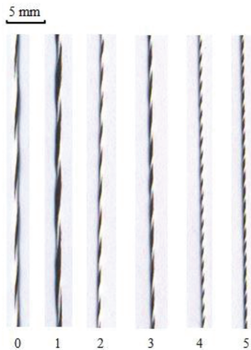
Figure 7 | Different classes of coded yarn specimens, where the annotated number indicates the digit represented by each coded yarn class.
