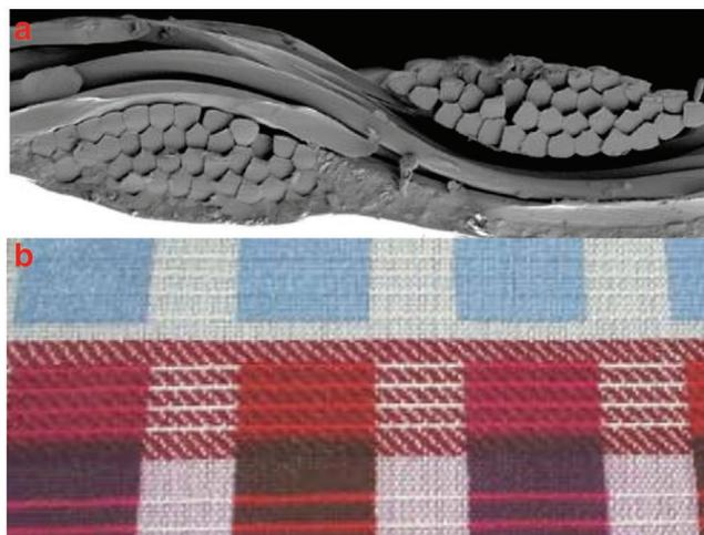
**Figure 7.** a) Cross-section of woven fabric. Reproduced with permission.<sup>[28]</sup> Copyright 2018, MDPI. b) Photograph of the woven optoelectronic fabric. Reproduced with permission.<sup>[153]</sup> Copyright 2013, Elsevier.
