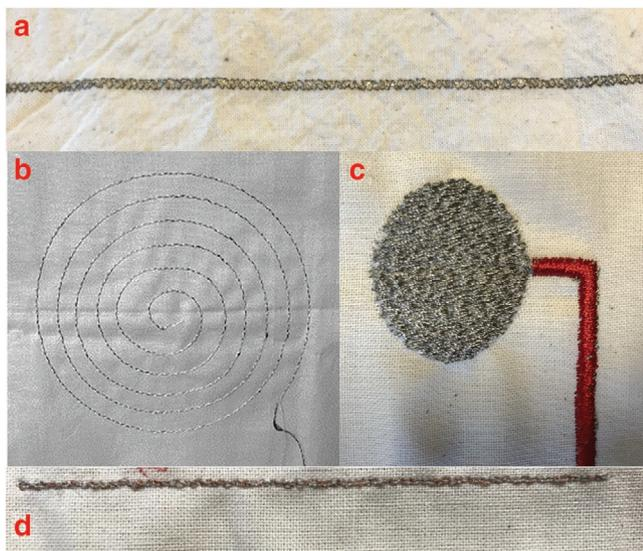
**Figure 5.** a) Embroidered silver yarn on the fabric. b) Embroidered stainless steel yarn as an antenna. Reproduced with permission.<sup>[124]</sup> Copyright 2004, Elsevier. c) Embroidered textile electrode for ECG measurements. d) Embroidered copper yarns.
