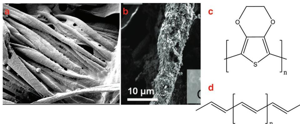
**Figure 1.** SEM image of cotton fibers with PEDOT:PSS coating. Reproduced with permission.<sup>[28]</sup> Copyright 2018, MDPI. b) SEM image of PANI and carbon-coated yarns. Reproduced with permission.<sup>[29]</sup> Copyright 2016, Springer Nature. Chemical structure of c) PEDOT and d) polyacetylene.
