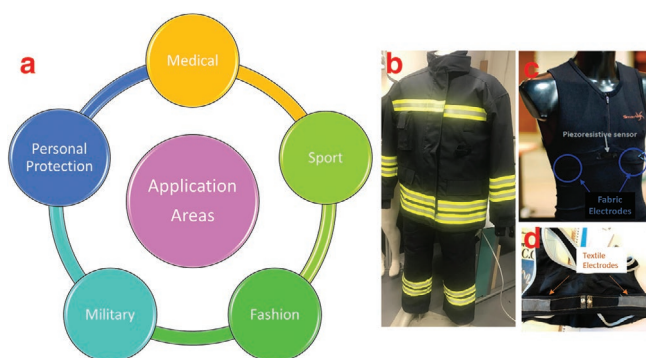
Figure 8. a) Main application areas of wearable electronic textiles. b) Fire-fighter suit equipped with emergency response sensors. c) Wearable piezoresistive sensors and fabric electrodes. Reproduced with permission. [193] Copyright 2016, MDPI. d) Image of the wearable knitted electrodes for the measurement of ECG signal. Reproduced with permission. [167] Copyright 2018, MDPI.
