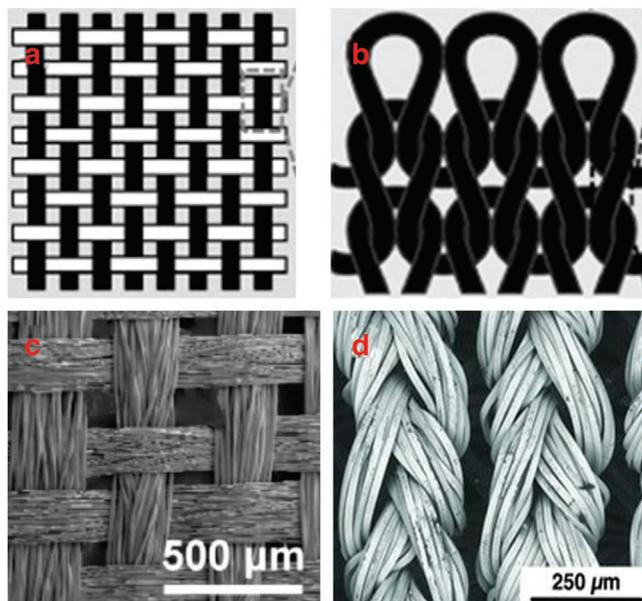
**Figure 3.** Schematic representations of a) woven and b) knitted fabric constructions. Reproduced with permission.<sup>[83]</sup> Copyright 2017, Elsevier. c) The morphology of the nickel-coated woven fabric. Reproduced with permission.<sup>[84]</sup> Copyright 2013, American Chemical Society. d) Knitted fabric containing silver-coated polyamide yarns. Reproduced with permission.<sup>[85]</sup> Copyright 2012, John Wiley and Sons.
