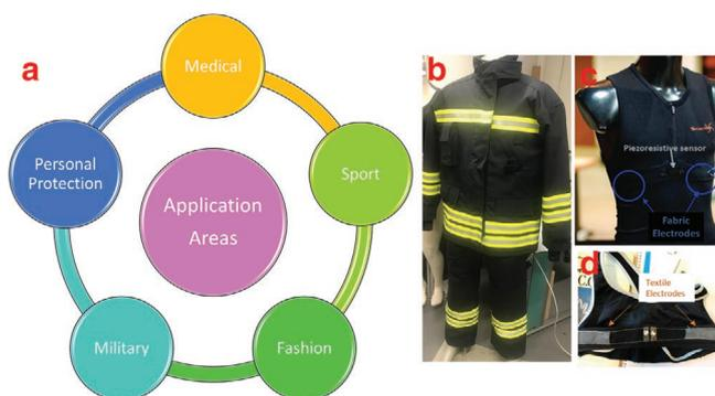
**Figure 8.** a) Main application areas of wearable electronic textiles. b) Fire-fighter suit equipped with emergency response sensors. c) Wearable piezoresistive sensors and fabric electrodes. Reproduced with permission.<sup>[193]</sup> Copyright 2016, MDPI. d) Image of the wearable knitted electrodes for the measurement of ECG signal. Reproduced with permission.<sup>[167]</sup> Copyright 2018, MDPI.
