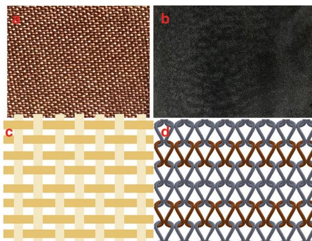
**Figure 4.** a) Photograph of Ni/Cu coated woven fabric. b) Photograph of PEDOT:PSS dip-coated knitted cotton fabric. c) Basic weaving structure. d) Representation of knitted elastomeric and conductive yarn. Reproduced with permission.<sup>[110]</sup> Copyright 2013, MDPI.
