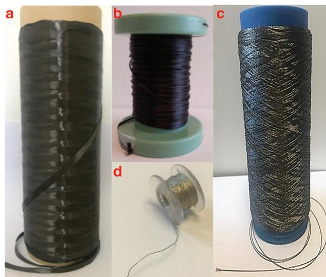
**Figure 2.** Conductive yarns: a) Carbon fiber, b) carbon-nanotube-containing yarn. Reproduced with permission.<sup>[51]</sup> Copyright 2014, Elsevier. c) Stainless steel yarn, d) silver-coated polyamide yarn.
