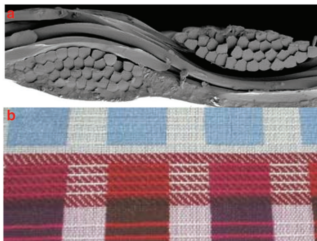
Figure 7. a) Cross-section of woven fabric. Reproduced with permission. [28] Copyright 2018, MDPI. b) Photograph of the woven optoelectronic fabric. Reproduced with permission. [153] Copyright 2013, Elsevier.
