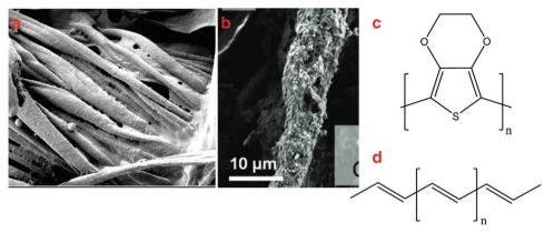
Figure 1. SEM image of cotton fibers with PEDOT:PSS coating. Reproduced with permission.<sup>[28]</sup> Copyright 2018, MDPI. b) SEM image of PANI and carbon-coated yarns. Reproduced with permission.<sup>[29]</sup> Copyright 2016, Springer Nature. Chemical structure of c) PEDOT and d) polyacetylene.
