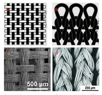
**Figure 3.** Schematic representations of a) woven and b) knitted fabric constructions. Reproduced with permission. [83] Copyright 2017, Elsevier. c) The morphology of the nickel-coated woven fabric. Reproduced with permission. [84] Copyright 2013, American Chemical Society. d) Knitted fabric containing silver-coated polyamide yarns. Reproduced with permission. [85] Copyright 2012, John Wiley and Sons.
