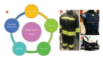
Figure 8. a) Main application areas of wearable electronic textiles. b) Firefighter suit equipped with emergency response sensors. c) Wearable piezoresistive sensors and fabric electrodes. Reproduced with permission. [193] Copyright 2016, MDPI. d) Image of the wearable knitted electrodes for the measurement of ECG signal. Reproduced with permission. [167] Copyright 2018, MDPI.
