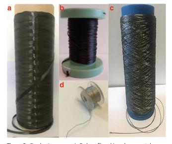
**Figure 2.** Conductive yarns: a) Carbon fiber, b) carbon-nanotube-containing yarn. Reproduced with permission.<sup>[51]</sup> Copyright 2014, Elsevier. c) Stainless steel yarn, d) silver-coated polyamide yarn.
