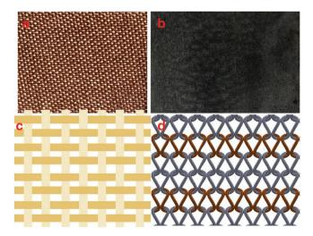
Figure 4. a) Photograph of Ni/Cu coated woven fabric. b) Photograph of PEDOT:PSS dip-coated knitted cotton fabric. c) Basic weaving structure. d) Representation of knitted elastomeric and conductive yarn. Reproduced with permission.[110] Copyright 2013, MDPI.
