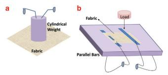
Figure 6. Schematic diagram of resistance measurement: a) cylindrical weight, b) parallel bars methods.
