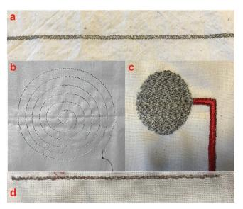
**Figure 5.** a) Embroidered silver yarn on the fabric. b) Embroidered stainless steel yarn as an antenna. Reproduced with permission. [124] Copyright 2004, Elsevier. c) Embroidered textile electrode for ECG measurements. d) Embroidered copper yarns.
