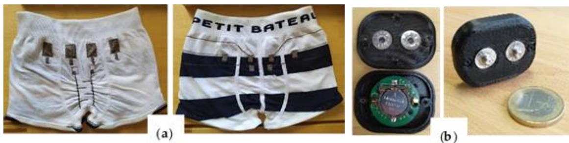
Figure 3. (a) Trunk integrating leakage sensor; and (b) photographs of the electronic module.
