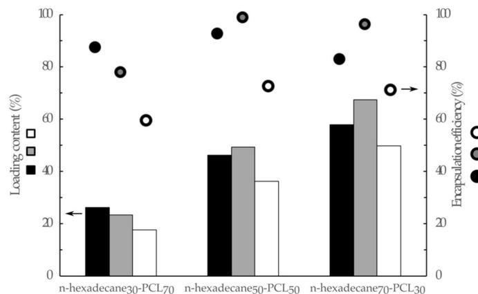
**Figure 4.** Influence of the nozzle system and the concentration of the PCL solution on the loading content and encapsulation efficiency (black—coaxial nozzle—5 w/v % PCL; grey—coaxial nozzle—10 w/v % PCL; white—single nozzle—10 w/v % PCL).
