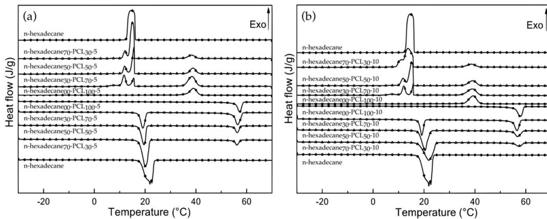
**Figure 3.** DSC thermograms of raw n-hexadecane, neat PCL microparticles and a series of n-hexadecane/PCL microcapsules obtained from PCL concentrations at 5 (a) and 10 (b) w/v % with different loading ratios between n-hexadecane and PCL.
