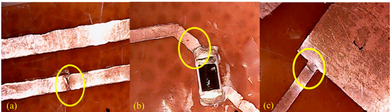
Figure 11. Damage analyses of washed PCBs with an optical microscope: (a) cracks in the track lines; (b) cracks at SMD pasting point; (c) cracks at the joint position of track lines and measuring pad.
