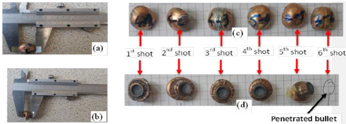
Figure 9. Recovered projectile debris diameter and length measurements (a,b) measurement system (c,d). Images of the recovered projectile debris after armour panel test.
