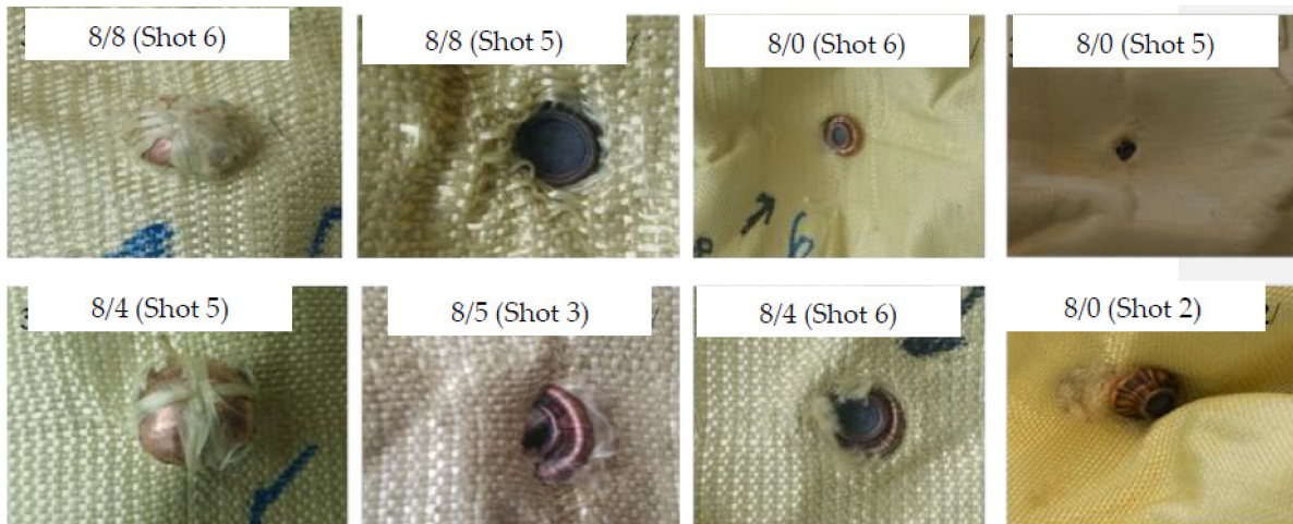
Figure 5. Some trapped projectiles inside the armour panel system.
