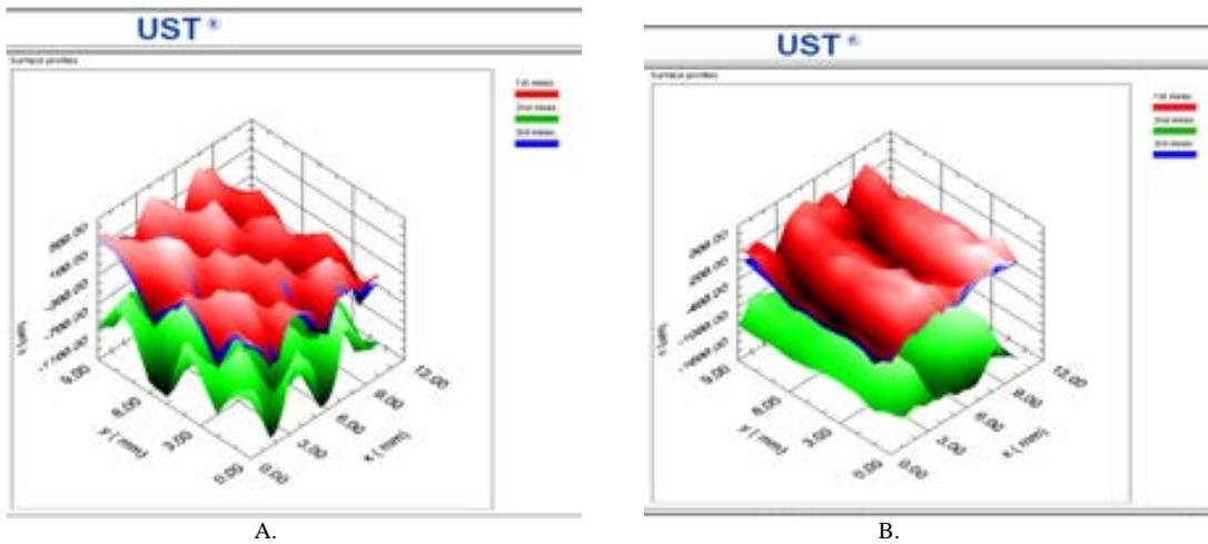
FIGURE 2. Polymer fibrous knitted matrix T2: A) 3D image obtained with UST, using ball sensor (X<sub>AXIS</sub> 0-9 mm, Y<sub>AXIS</sub> 0-8 mm, Z<sub>AXIS</sub> 200 to -1200 μm); B) 3D image obtained with UST, using papillary sensor. (X<sub>AXIS</sub> 0-12 mm, Y<sub>AXIS</sub> 0-9 mm, Z<sub>AXIS</sub> 400 to -1200 μm).
