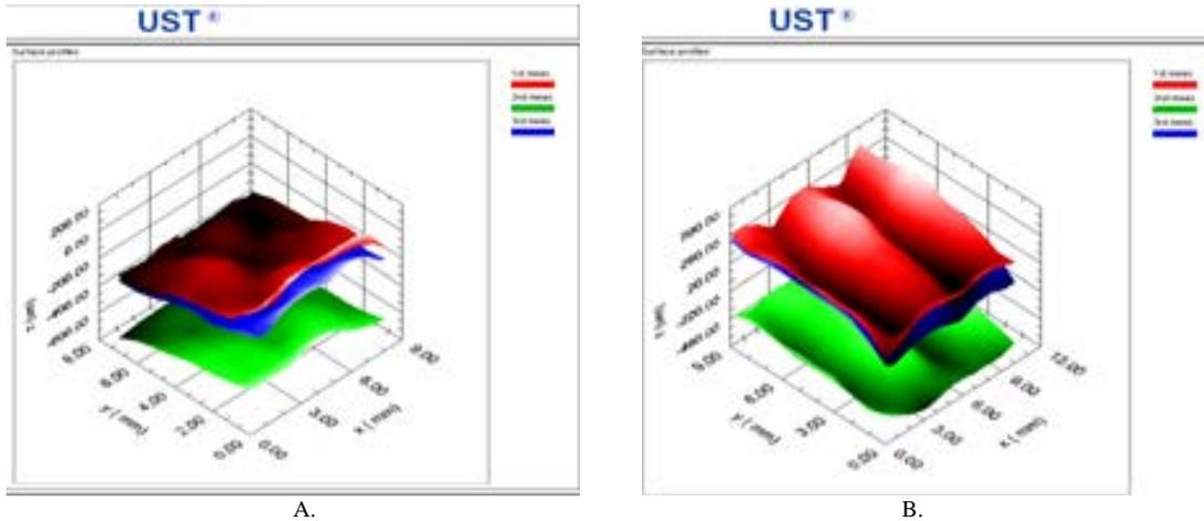
FIGURE 1. Polymer fibrous knitted matrix T1: A) 3D image obtained with UST, using ball sensor (X<sub>AXIS</sub> 0-9 mm, Y<sub>AXIS</sub> 0-8 mm, Z<sub>AXIS</sub> 200 to -800 μm); B) 3D image obtained with UST, using papillary sensor. (X<sub>AXIS</sub> 0-12 mm, Y<sub>AXIS</sub> 0-9 mm, Z<sub>AXIS</sub> 400 to -600 μm).
