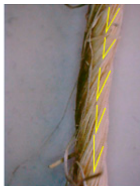
Figure 9. Sisal yarn with measurement for twist angle by ImageJ software (experimental method).
