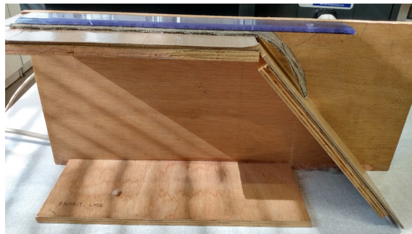
Figure 3. Cantilever test bench.
