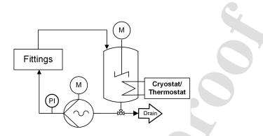
Figure 1: Process flow diagram of the test rig used to generate the investigated data set [53].
