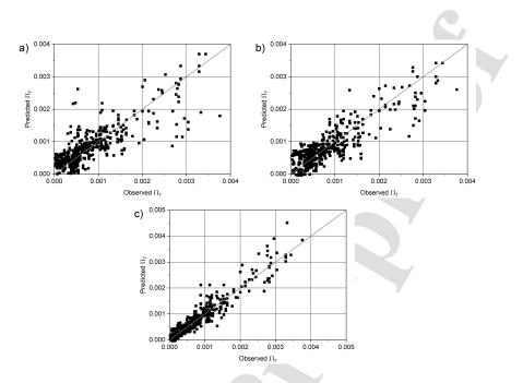
Figure 5: Measured vs. predicted plots for the combination of socket and bend for a) LR, b) SR and c) RF applying the set of dimensionless numbers.
