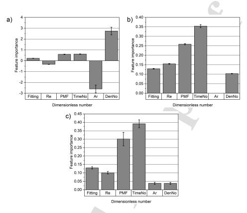
Figure 4: Calculated feature importance by a) LR, b) SR and c) RF applying the combined data set of socket and bend for dimensionless numbers.
