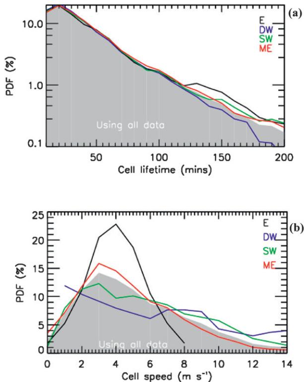
FIG. 5. As in Fig. 3a, but showing the PDFs of TITAN (a) cell lifetime using a bin size of 10 min in time and (b) cell speed using a bin size of  $1 \text{ m s}^{-1}$  for the respective large-scale atmospheric regimes. As discussed in the text, only TITAN cells with lifetimes  $> 10$  min (and cells that formed and decayed within 140 km of the radar center) are used in this figure and all subsequent figures.
