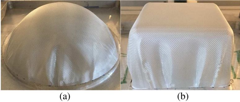
Fig. 11. Wrinkling phenomenon in (a) hemispherical and (b) square-box forming.
