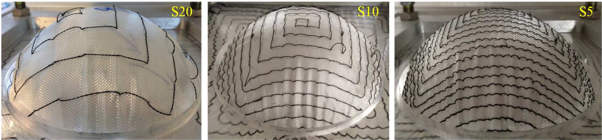
(a) Forming of the tufted preforms with the square spiral pattern
