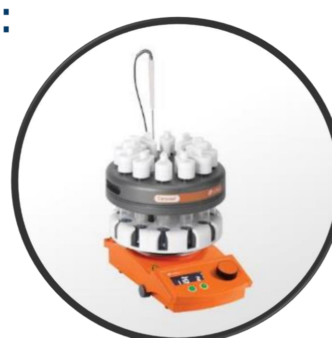
Radleys carousel (12 reactors)
