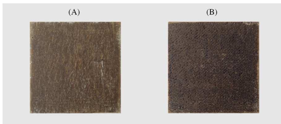
FIGURE 1 (A) PLLA/unidirectional flax(UD) and (B) PLLA/twill flax(TW) composite plates (120 × 120 mm).
