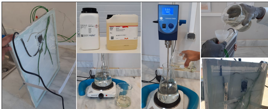
Fig. 3. PV panel system set up: covering the backside of the panel and filling the system with the melted PCM.
