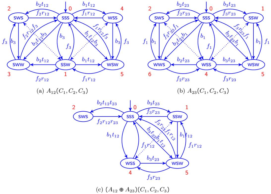
Figure 2.7: Projections of reachable states of the compound behaviours onto  $\sigma(A_{id}(C_1, C_2, C_3))$  (for ease of reading, I omit the transitions indicated by dotted blue arrows; furthermore, for ease of comparison between sub-figures, I additionally label each state with a red number, whereof the main label is the binary representation with  $\mathbf{s} = 0$  and  $\mathbf{w} = 1$ )
