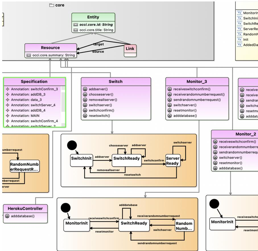
Figure 4.10: Fragment of the OCCIware design of *Monitor-Switch* Web application
