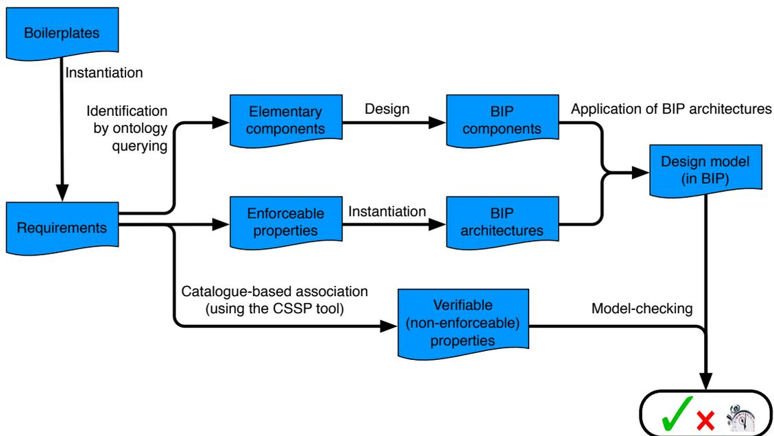
Figure 2.8: High-level illustration of the CSSP design process
